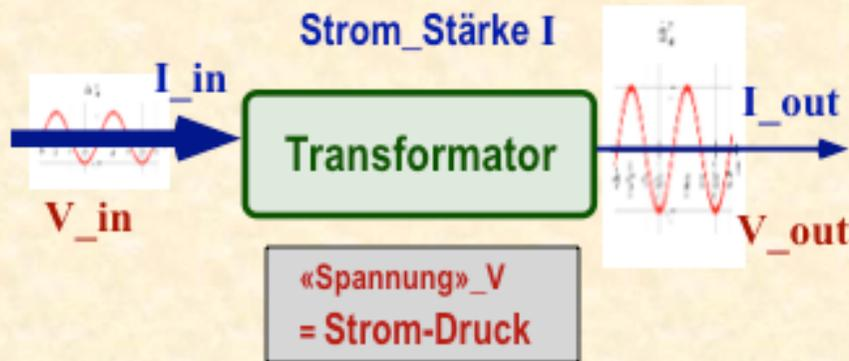
$$\text{Ideal: } I_{in} * V_{in} = I_{out} * V_{out}$$
